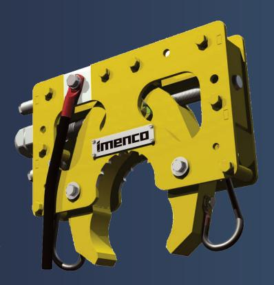
Two main benefits in choosing a Caiman Clamp™ are its ease of installation and versatility. It can be used to bond an anode sled to a structure or it can be installed with anodes directly attached. Slim form factor and low weight add to the flexibility and robustness of this design. The clamp is simply guided into place by a diver or ROV and tensioned with a torque tool to ensure a secure and low resistant connection.
